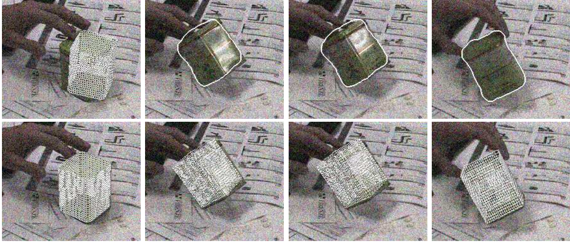
Figure 7: Top row: Initialization at the first frame. Contour at frames 49, 50, and 116 of the sequence. Bottom row: Pose results at frames 0, 49, 50, and 116. The tea box is moved, causing partially severe reflections on the box. Furthermore, Gaussian noise with standard deviation 30 has been added.
