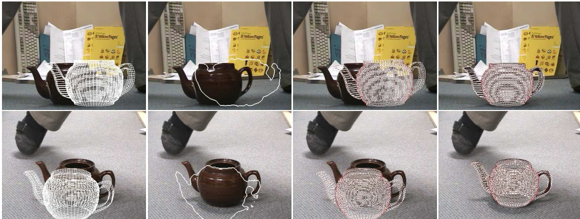
Figure 11: From left to right: (a) Stereo image with a teapot. The initialization is quite far away from the object. (b) Resulting contour when performing only one iteration. The contour is restricted to the initial, bad pose and cannot fully capture the object. (c) Consequently, the pose remains close to the initialization. (d) Pose result after 20 iterations.
