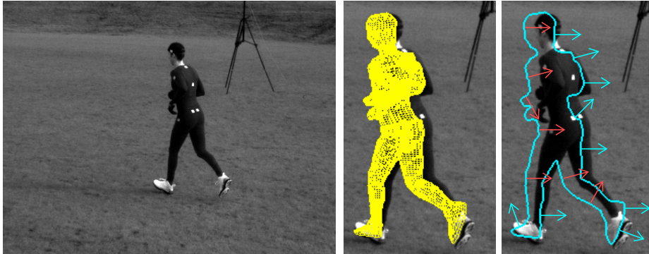
Fig. 1. This figure illustrates the movement applied to contour points by the tracking algorithm used. Left: Example input image of a scene. Middle: Object model projected in an inaccurate pose into the image plane (magnified). Right: Silhouette of the projected model and an example how some contour points might be adapted by the tracking algorithm (magnified). Cyan arrows indicate points that are moved towards the outside and red arrows indicates a movements towards the inside of the object.
