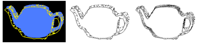
Fig. 4. Left: Projected object surface in blue and the extracted object contour in yellow. One seeks corresponding points between the silhouette of the blue area and the yellow contour. Center: Closest point correspondences. Right: Regularized closest point computed with optical flow numerics and \alpha = 10 .
