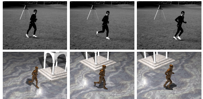
Fig. 15. Full body tracking in a sequence with ground truth data. Top row: Input frames from one out of four camera views. Bottom row: Synthesized images from the tracked 3D pose. A different viewpoint than in the input images is depicted. Further results are shown in Figures 16, 18, 17, and Table II.
