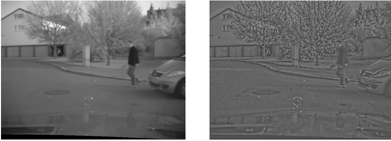
Fig. 5 An example of the residual images used as input to the scene flow algorithm in this paper. The original is on the left, with the residual processed image on the right.
