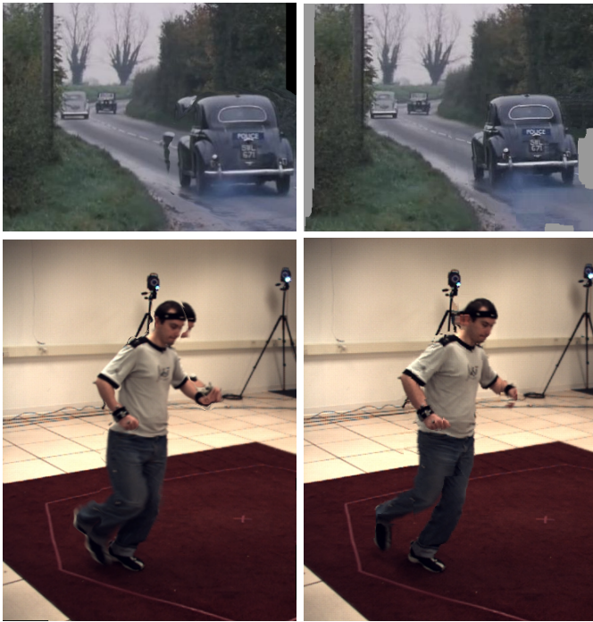
Fig. 7. Warped second image; see Fig. 6 for flow. Left: Large displacement optical flow. Right: SIFT flow. The SIFT flow warps look nicer as occluding structures are not doubled, but this reveals actual problems in the estimated flow (see text). Animations are available in the supplemental material.
