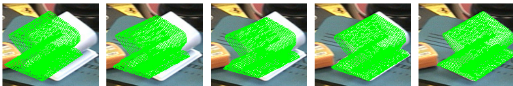
Figure 5: From left to right: Initial guess, and pose estimated after 10, 30, 50, and 70 iterations (magnified).
