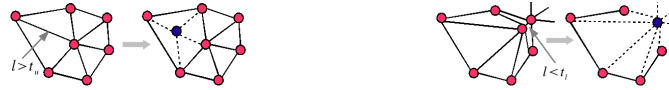
Figure 5.2.: (left) If the length l > t_u , the edge is split. (right) Edges for which l < t_l are merged.
