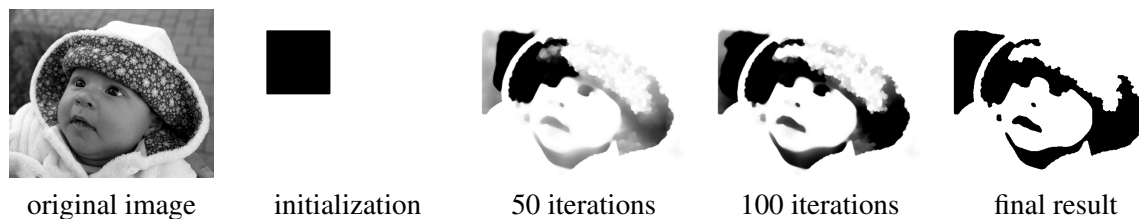
Figure 2.2.: Result of the convex region-based segmentation. The mean values \mu_1 and \mu_2 were set to 0.2 and 0.55 (on a scale of from 0 to 1) respectively, \lambda was set to 0.017.
