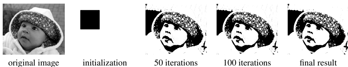
Figure 2.3.: Result of the convex geodesic active contour segmentation. The mean values \mu_1 and \mu_2 were set to 0.2 and 0.55 (on a scale from 0 to 1) respectively, \lambda was set to 2.5.
