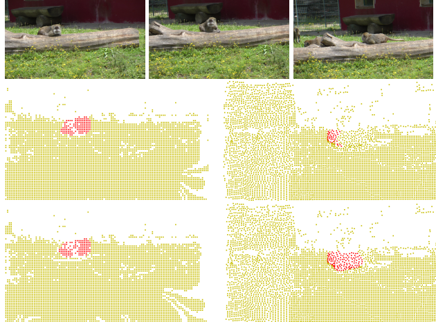
Figure 13. First row: Monkey that lies in the beginning, stands up, and turns to the other side. Second row: Result with pairwise affinities [4] for the first and last frame. Third row: Our result with 3-affinities. This examples shows that 3-affinities also better fit 3D rotations than pairwise affinities, though not explicitly modeled.
