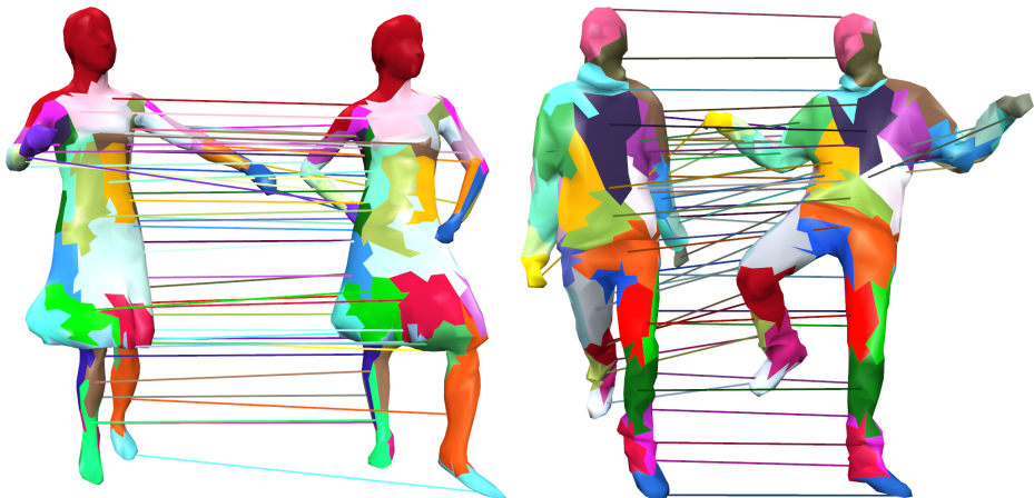
Fig. 1. Geometrically Consistent Elastic Matching. We propose to cast the dense elastic matching of surfaces in 3D as a codimension-two minimal surface problem which aims at minimizing the distortion when transforming one shape into the other. We show that a consistent discretization of this minimal surface problem gives rise to an integer linear program. By means of LP relaxation we can compute near-optimal matchings such as the one shown above. These matchings are dense triangle-wise matchings. (For visualization we combined triangles to patches and colored them consistently with their corresponding patch.)
