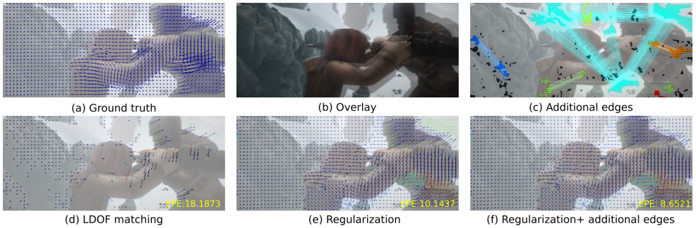
Figure 3: Benefit of additional edges. When matching the first frame to the second (b), we compute regions with little texture, highlighted as black and colored areas in (c). Noise and small regions are discarded (marked as black). The remaining regions are connected if their appearance is similar. Connected regions have the same color. The bottom row shows the improvement from the initial LDOF [1] correspondences (d), over the refined matches (e) to and the refinement with the extended set of edges (f). The arrows are colored from blue to red (small to high error).
