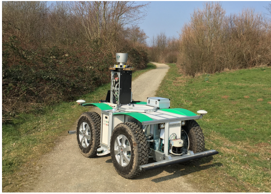
Fig. 3. The Viona autonomous mobile robot platform equipped with bumblebee stereo cameras and a modified dashcam with the NIR-cut filter removed.
