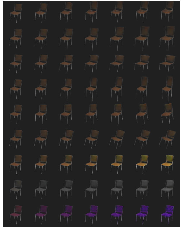
Fig. 22. The effect of specialized neurons in the layer FC4. Each row shows the result of increasing the value of a single FC4 neuron given the feature maps of a real chair. Effects of all neurons, top to bottom: translation upwards, zoom, stretch horizontally, stretch vertically, rotate counter-clockwise, rotate clockwise, increase saturation, decrease saturation, make violet.
