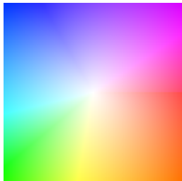
Figure 1. Flow field color coding used in this paper. The displacement of every pixel in this illustration is the vector from the center of the square to this pixel. The central pixel does not move. The value is scaled differently for different images to best visualize the most interesting range.
