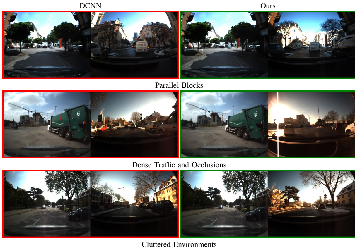
Fig. 7: The correct matches are shown in Green borders and the false matches are shown in Red . Our approach helps to diminish false matches by boosting features from stable image regions, suppressing spatial ambiguities and leveraging original DCNN activations.
