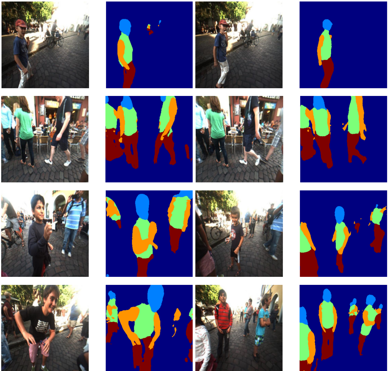
Fig. 13: Segmentation examples on multiple scenarios on Freiburg City Dataset. The first row presents segmentation of a single instance in a sequence. Second row exemplifies an example of segmentation for multiple instances in a sequence. The third and fourth rows show segmentation results under glare, occlusion and multiple instances presence.
