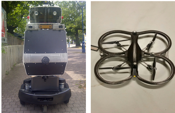
(a) Obelix ground robot. (b) AR.DRONE 2.0 aerial platform.
