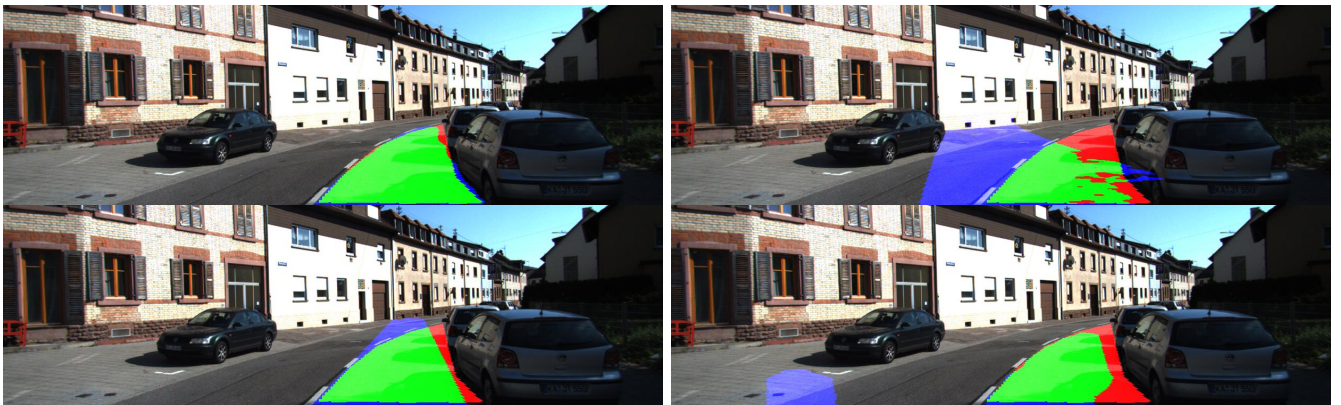
Fig. 9: Lane predictions on the KITTI dataset compared with the 3 next best approaches. Top Left: Fast-Net, Top Right: ANN, Bottom Left: PCA-Lane-S, Bottom Right: S. In the images green is the correct segmentation, red false negative detection and blue false positive detection.
