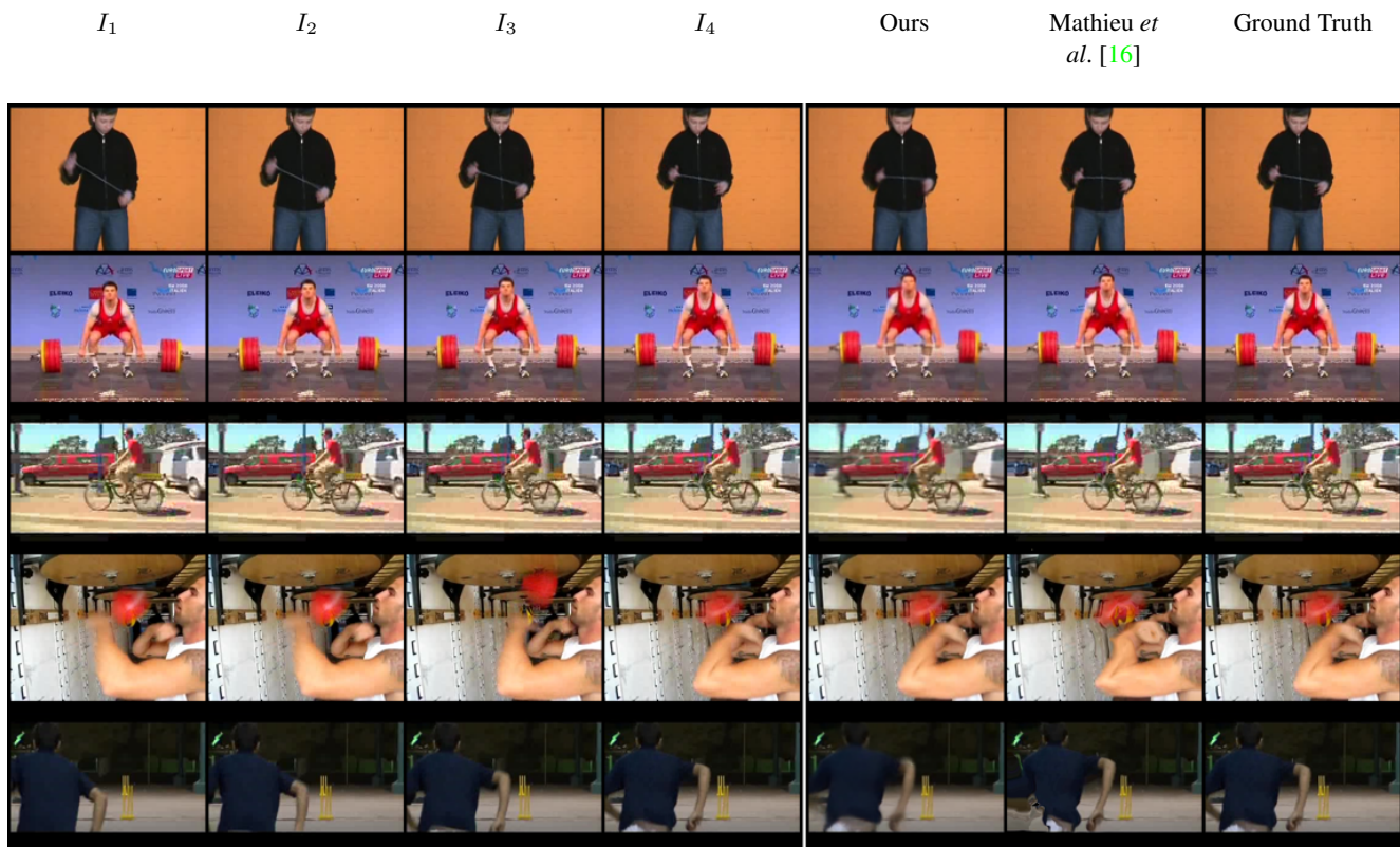
Figure 7: Next frame prediction samples. Results of Mathieu et al. [16] are often a bit sharper due to the adversarial loss, yet the method also introduces distortions and artifacts; see the last two samples. Our next frame predictions are blurrier due to relying only on the L1 loss, but yield robust predictions without distortion. This explains the on-par quantitative results in Table 4.
