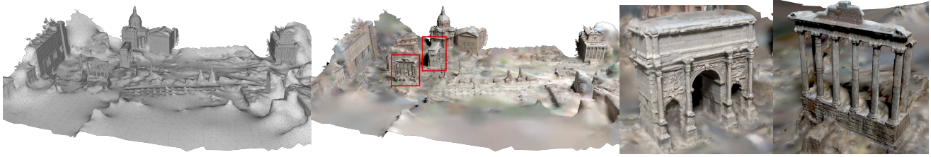
Figure 13. Dense reconstruction of the roman forum with our method. The input point cloud contains 638 million samples. Left: Wireframe rendering. Sights like the arch have a very high resolution in the octree and in the resulting surface mesh. The density of the triangle mesh changes smoothly due to the balancing criterion we imposed on the octree. Center: Colored reconstruction. Right: Close-up of the arch and temple.
