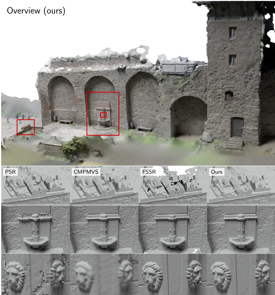
Figure 10. Reconstruction of the Citywall data set from (Fuhrmann et al, 2014) with 256 million points. Overview: Colored reconstruction of the whole scene with our method. The annotations mark the three close-up views which are (top to bottom) the city model, the fountain and the lion heads. PSR: The reconstruction with PSR contains many noise artifacts. Some artifacts could be removed with the provided clean-up tool in exchange for causing holes in the reconstruction as seen in the city model. The reconstruction of the lion heads is too smooth due to a maximum octree depth of 14. Memory limits did not permit a reconstruction using a deeper octree. CMPMVS: The CMPMVS software correctly models most of the empty space between the houses in the city model. Some surfaces near the fountain show noise artifacts and seem to model noise. The resolution of the underlying tetrahedral net was chosen too coarse to reconstruct the lion heads with all details. Note that the CMPMVS software computes its own depth maps at full image resolution to generate its own input point cloud. FSSR: FSSR generates a detailed reconstruction of the scene but has problems with holes in the city model and shows artifacts in the basin of the fountain. The artifacts are linked with the rest of the scene and cannot be removed easily. Of all methods, FSSR shows the best reconstruction near the mouths of the lion heads. Ours: Our method generates a surface without holes for the city model and preserves most of the concave structure between the houses. The basin of the fountain has some small artifacts. In contrast to FSSR, the view to the bottom of the basin is not blocked by reconstruction artifacts. The lion heads show all details but the surface of the taps of the lions is slightly underestimated. We set \lambda_{1,2} = 1 , \alpha_{1,2} = 2 for this data set. Results for SSD are not shown because the method did not finish after multiple days.
