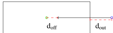
Fig. 5. Pixel-to-Box Assignment: Each pixel (blue circle) predicts an offset vector (black arrow) towards an object center (black rectangle with green circle). If the pixel lies outside of a predicted box, it is punished with the distance to the closest box boundary d_{\text{out}} . Additionally, the difference between offset prediction and box center is punished with d_{\text{off}} .
