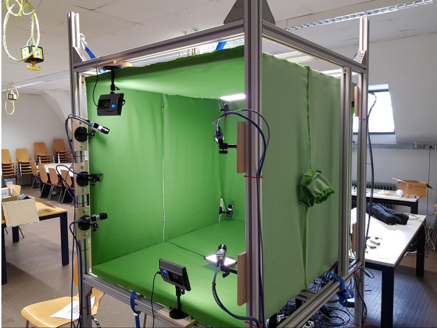
Figure 3: Recording setup with 8 calibrated and temporally synchronized RGB cameras located at the corners of a cube. A green screen background can be mounted into the setup, enabling easier background subtraction.
