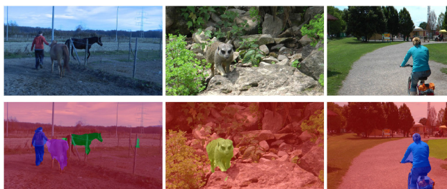
Fig. 5. Examples of CCC segmentation results densified by the variational method of Ochs et al. [52] on three sequences of the FBMS59 [54] benchmark.
