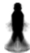
Fig. 8. The average pedestrian shape template used for the computation of pairwise terms between pedestrian detections and trajectories.
