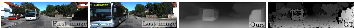
Fig. 11 Failure example on KITTI. Ours uses a sequence of 5 frames from the left color camera; the first and last frame are shown above. Our cost-volume-based approach suffers from the moving object (the silver bus in this example) and the occlusion (trees occluded by the bus).
