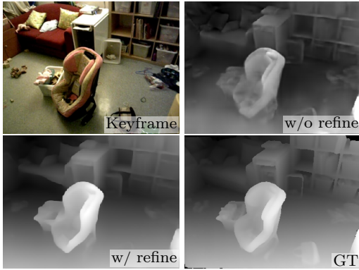
Fig. 4 Effects of the narrow band refinement. We apply the narrow band module for 15 iterations with and without refinement. Without the refinement, the module lacks the knowledge of the band shape and it can only make updates based on the measurements in the cost volume. This can help in capturing more details, but also causes strong artifacts. Appending a refinement network with previous depth estimation as input allows for a better regularized and more stable depth estimation.
