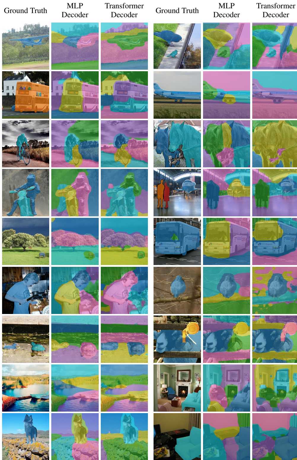
Figure 22: Masks on PASCAL VOC 2012 produced by our method, using 6 slots and a ViT-B/16 encoder. We show predictions from the MLP and the Transformer decoder.
