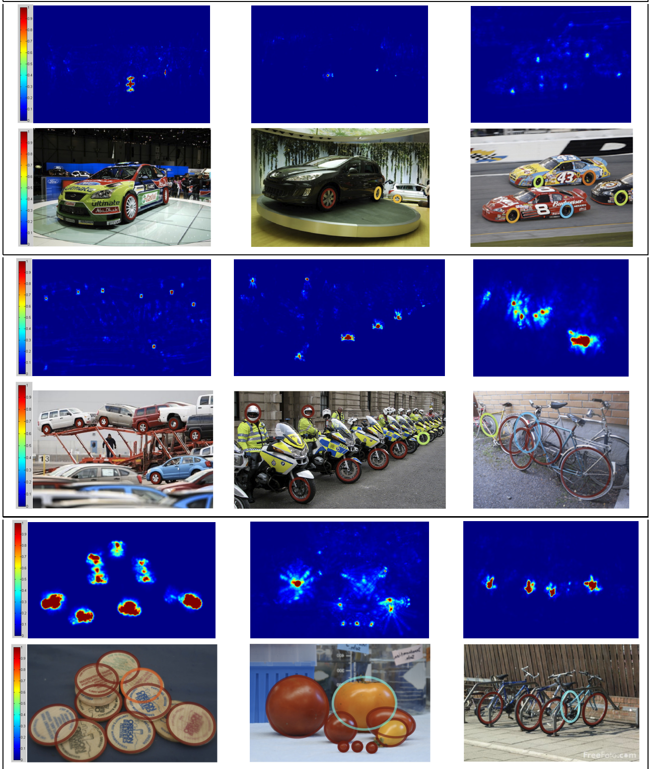
Figure 2. GFRS applied to real world images. Each pair of images shows the GFRS response map and the most confident detections corresponding to ellipses after thresholding the GFRS response map and non-maximum suppression.
