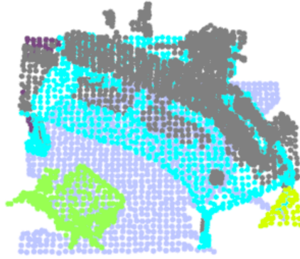
Figure 27: Proposed region for a table (cyan). The main direction of the table is not aligned with the coordinate system. Therefore the table cannot be extracted without the chair (green).
