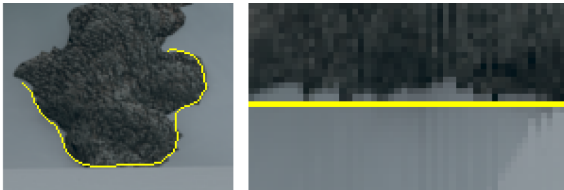
Figure 2.3: Boundary segments (yellow) from original images ( left ) are transformed into straight lines and images are warped respectively. Warped images ( right ) are then used for descriptor computation.
