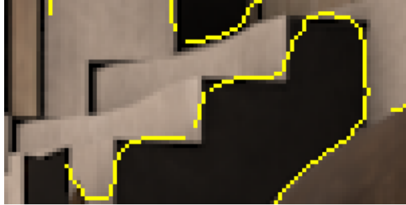
Figure 3.2: Boundaries estimated by Gb can significantly deviate from the actual boundaries in the image.
