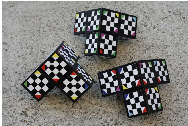
Fig. 1: The three calibration bodies, each consisting of 18 checkerboards in different orientations. The checkerboards facing down can be used in setups where the bodies are placed on a glass pane with cameras filming from below.
